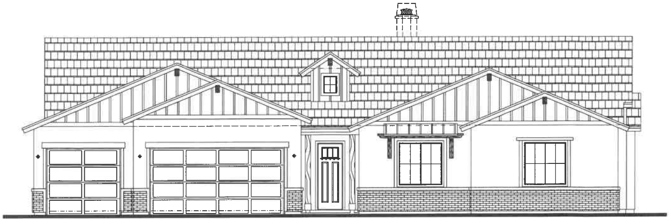
Elevation A - Front (Front Load Garage)
